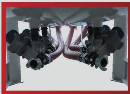
AUTOMATIC VALVE SYSTEM
